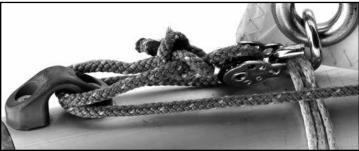
*Tip:* Spray boom with dry lubricant like McLube<sup>®</sup> to make outhaul adjustment easier.
